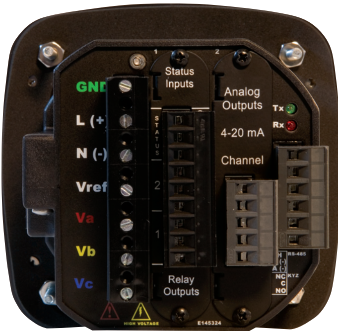
IQ 250/260 Meter (Rear View) With Connection and Communication Ports
